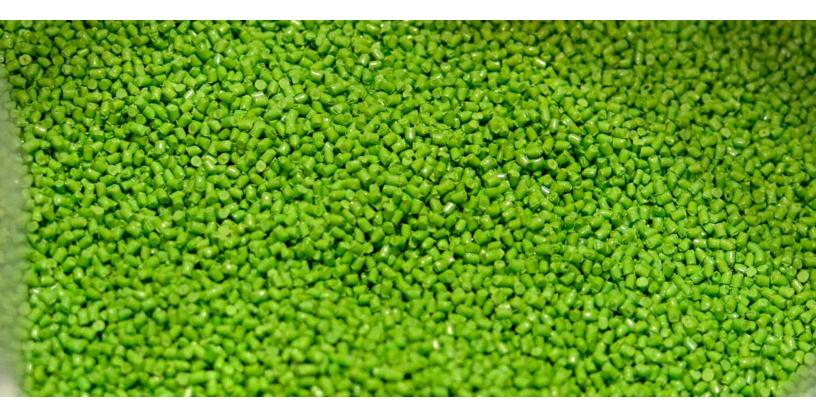
LCPs, or Liquid Crystal Polymers, are a unique class of thermoplastic resins, which are extremely non-reactive and inert. LCP is an expensive material that provides high performance for specialized, end-use applications, but it is not necessarily easy to work with. This paper will explore some of the potential pitfalls, and offer suggestions, solutions and best practices for working with the thermoplastic injection molding grades.
